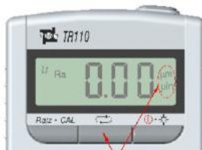
Switch the m/in by keep pressing the Middle Key.
