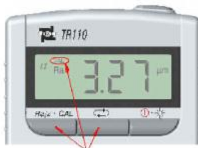
Under CAL status, press the Left Key to increase the value by turns and press the Middle Key to decrease the value.
