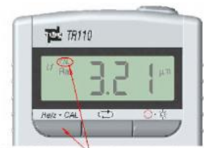
Press the Left Key for a long time, the tester will enter the status of Mean Value calibration and a symbol CAL will display on screen
