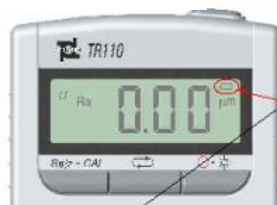
The symbol will appear when low battery, and it will twinkle during recharging
